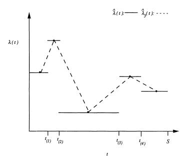
FIGURE 7. Piecewise-Linear Intensity Function  $\hat{\lambda}_3(t)$  When n = 4.
